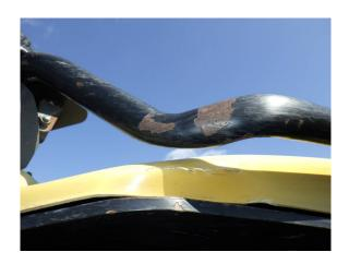
Hood THE TOP COVER IS WARPED AND WORN OUT
